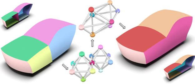
**Figure 10:** Left: Subvolumes and the surface graph. Right: Surface blending and merging produce a single abstraction shell.
