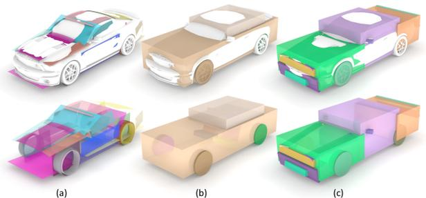
**Figure 5:** (a) RANSAC primitives based on surfaces, (b) Volumetric segmentation of [Attene et al. 2006] -the disconnected parts in the input mesh are manually stitched into a single mesh prior to processing in (b)- (c) Our basic primitives based on volumes.
