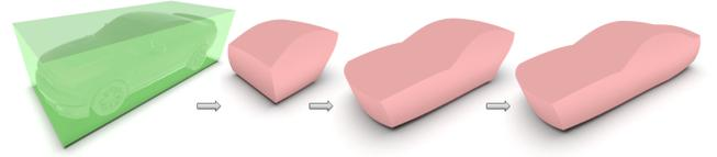
**Figure 11:** Starting from the bounding box, the simplest abstraction is found in multiple subvolume extraction steps.
