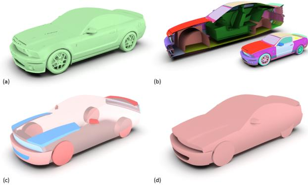
**Figure 7:** (a,b) The original model consists of many isolated components, together with components inside the volume. (c) A snapshot of our abstraction process with the current abstraction in light red. Positive (dark red) and negative (blue) subvolumes are identified in multiple consecutive steps. (d) The resulting abstraction when these subvolumes are applied.
