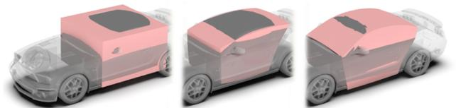
**Figure 9:** (a) A basic primitive. (b) Its surfaces are beautified using conventional regression. (c) The same surfaces beautified using our approach results in a more faithful representation of the original geometry.
